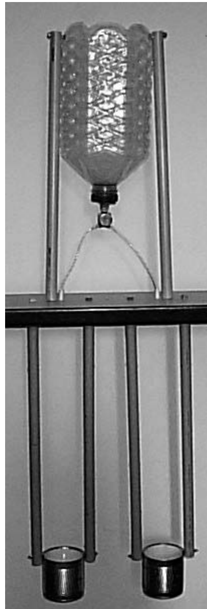
Fig. 8: The common form of electrostatic generator with the magnetic separation of the charges
