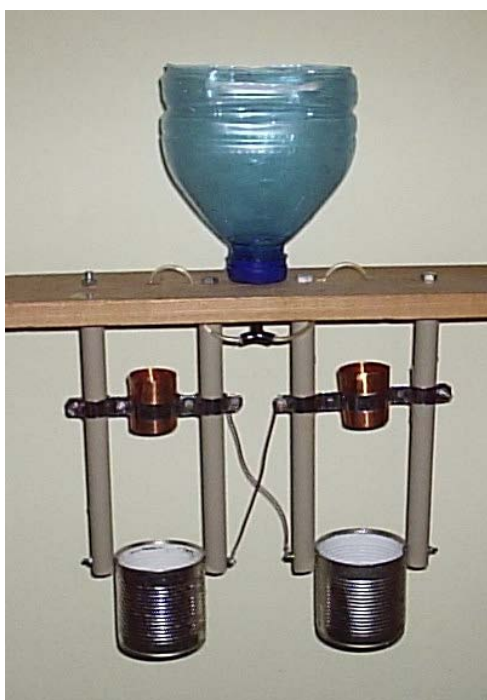
Fig. 6: The experimental layout of the Kelvin dropper
