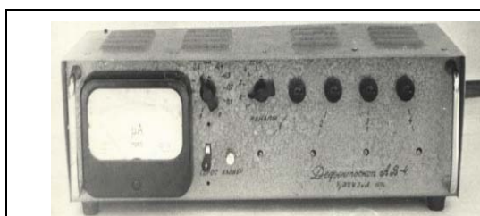
Figure 6: 4-channel acoustic-high-frequency device for monitoring the status of high voltage transformers
