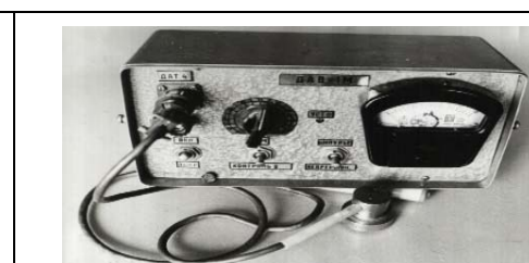
Figure 7: Single-channel acoustic-high-frequency device for monitoring the state of insulation high voltage transformers
