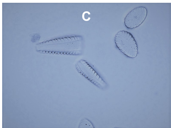
Figure 2: SEM micrograph of the: C - Non-activated sample algae Surirella and activated sample sulphide concentrate, D - Mechanochemical activated sample (sulphide concentrate and algae Surirella), gold nanoparticles attached in algal cells
