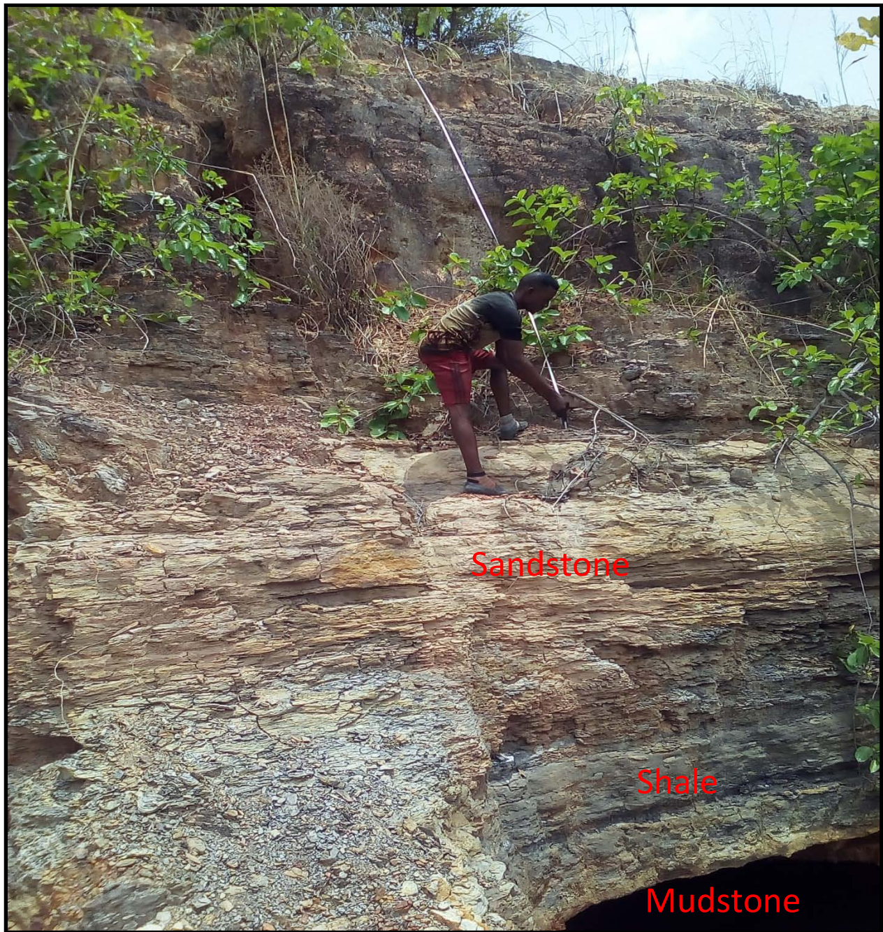
Fig. 3: Stratigraphic Section of Odagbo Coal Mine
