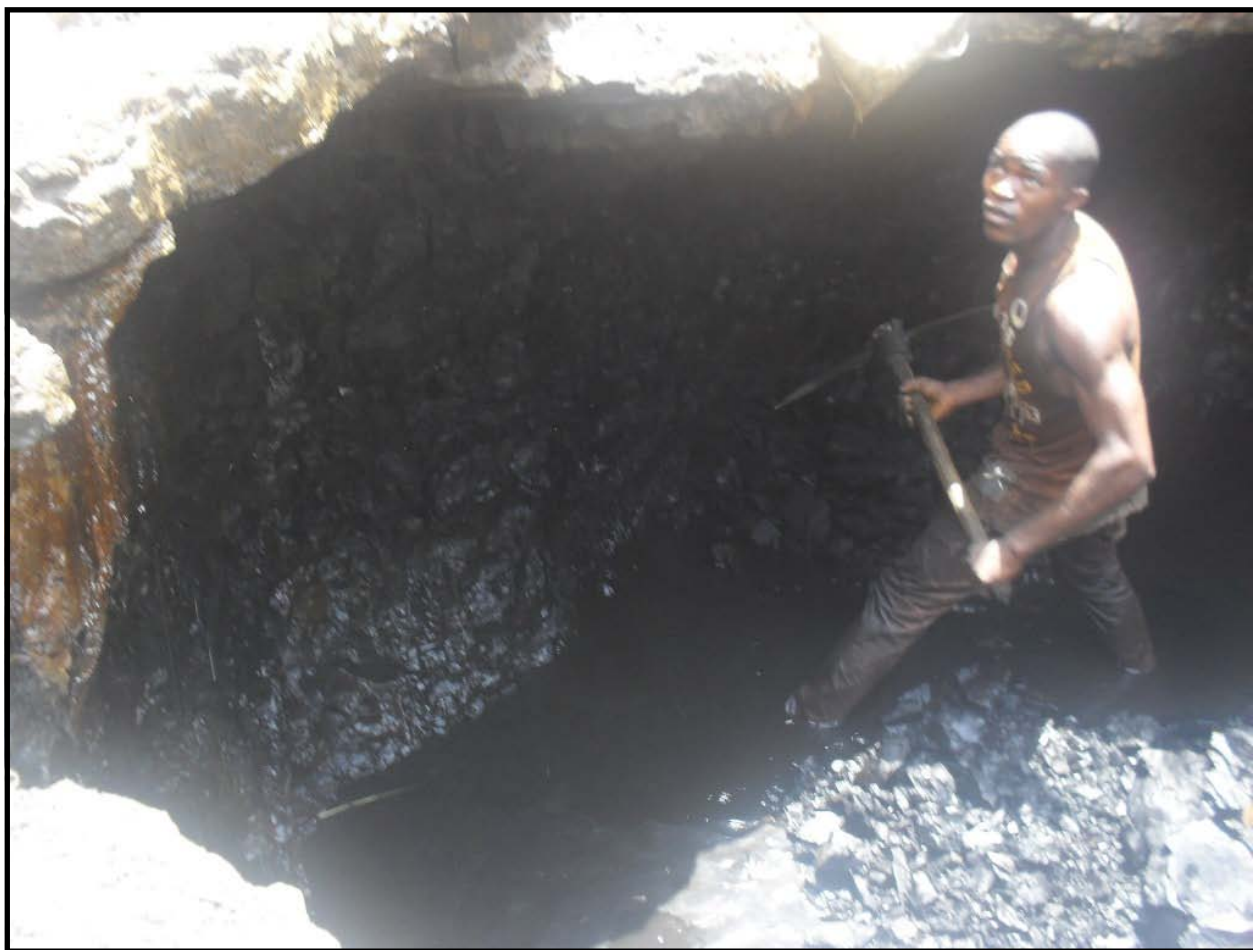
Fig. 1: An Artisanal Miner using a digger to excavate a Coal Seam
