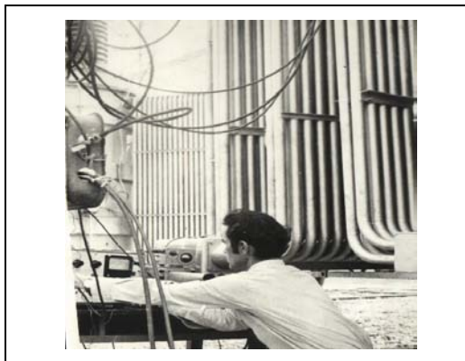
Figure 2: The process of studying partial discharges in transformers under operating conditions
