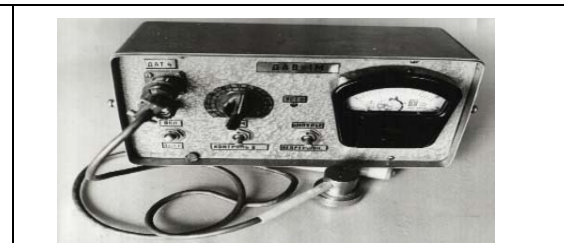
Figure 7: Single-channel acoustic-high-frequency device for monitoring the state of insulation high voltage transformers
