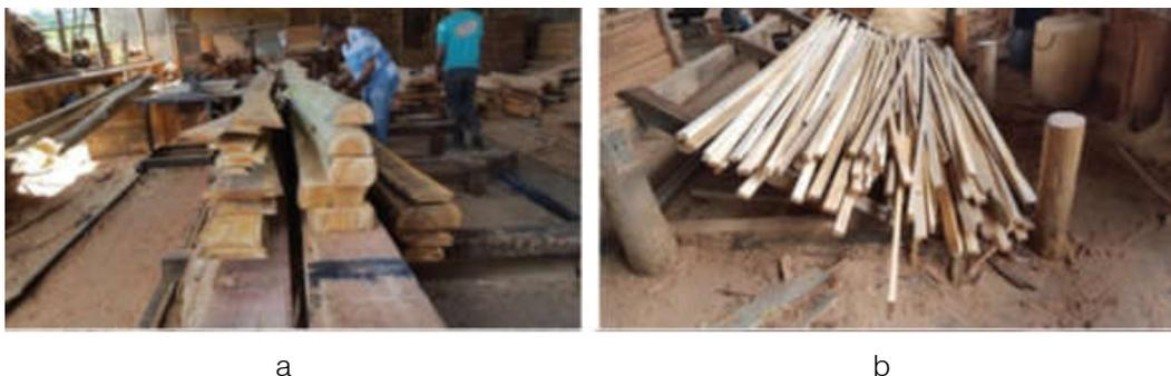
Fig. 6: a) First product of the longitudinal cut pattern and b) clapboards after the second step in a circular blade
