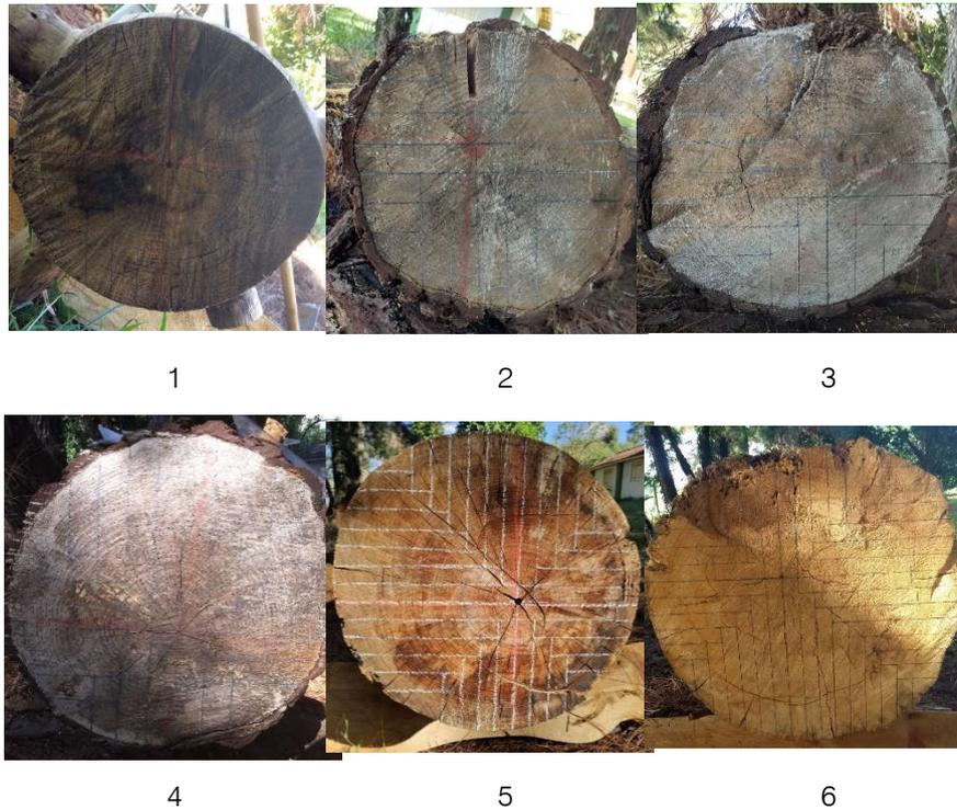
Fig. 15: Designed sections of Logs 1–6 with pieces of thickness 32 mm (27 + 5 mm) and width  $\geq 50$  mm and marrow bias of 2 cm (log 1); 4 cm (log 2); 4.5 cm (log 3); 5.3 cm (log 4); 6 cm (log 5) and 6.5 cm (log 6)
