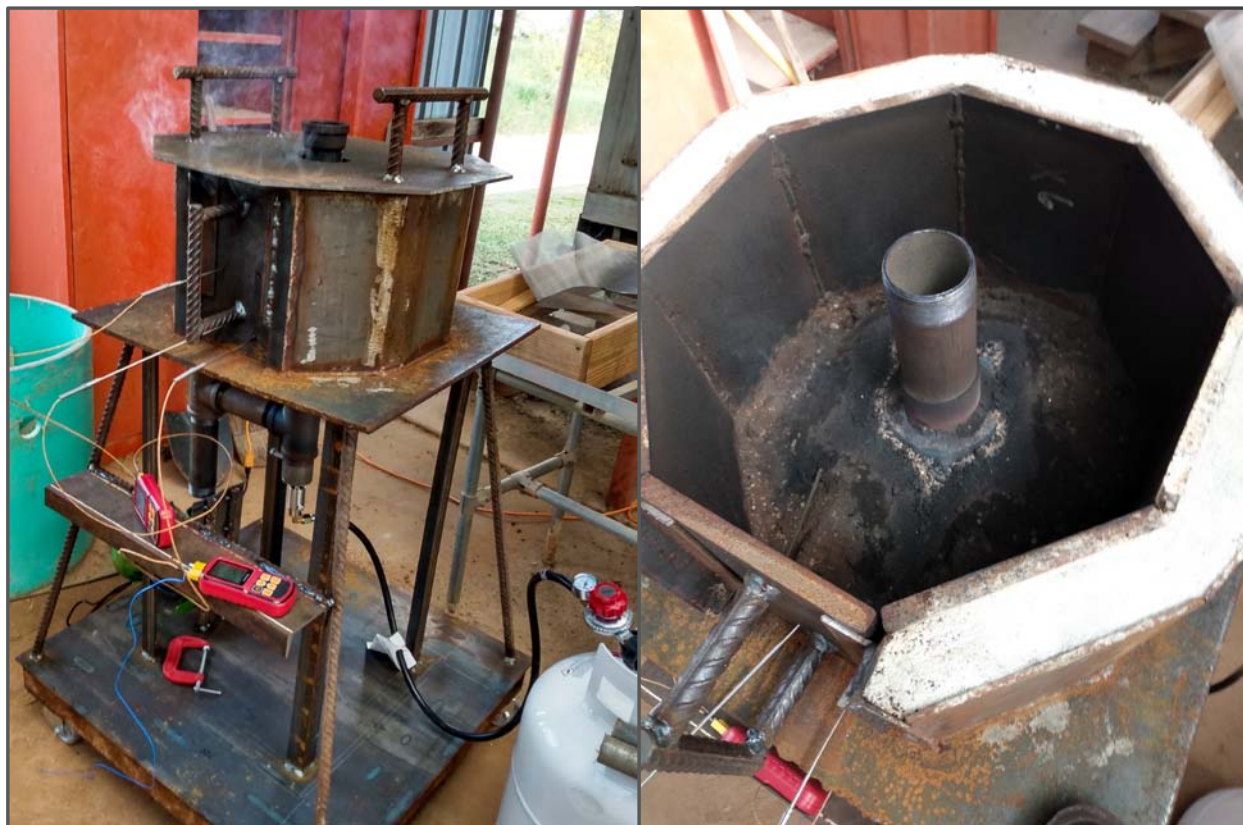
Figure 1: Image of smolder apparatus employed in study. Left image shows exterior with temperature probes in use. Right image shows interior of smolder chamber
