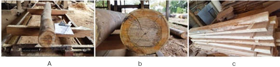
Fig. 4: a) Log in the sawmill machine, b) smaller face of a log with pieces calculated and selected to be cut, and c) stacked pieces to dry after measurement and identification
