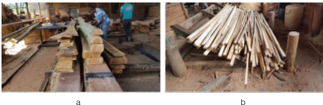
Fig. 6: a) First product of the longitudinal cut pattern and b) clapboards after the second step in a circular blade
