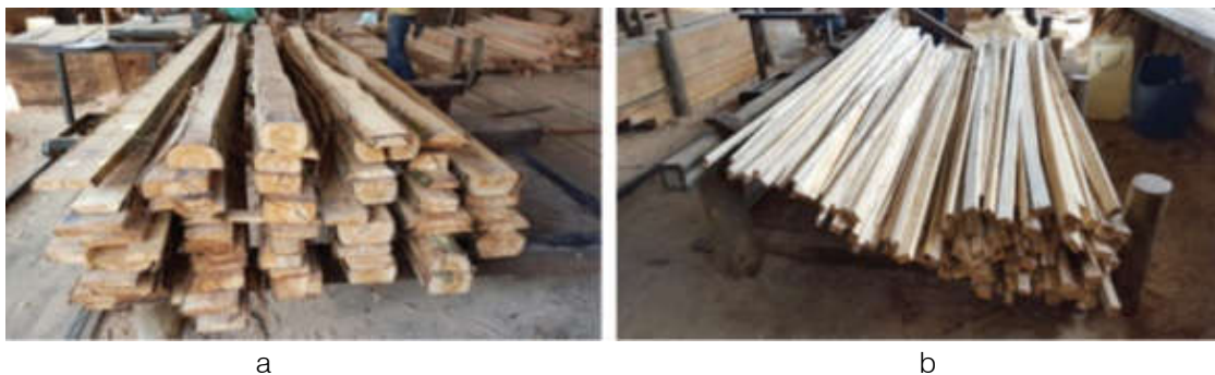
Fig. 5: a) First product of the empirical procedure and b) large clapboards and clapboards after going through the second step in a circular blade
