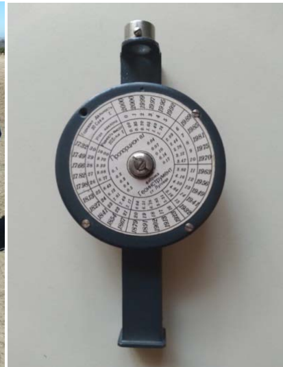
Fig. 7: The Device Measuring the Angle of Inclination of the "Eklimeter" Brand
