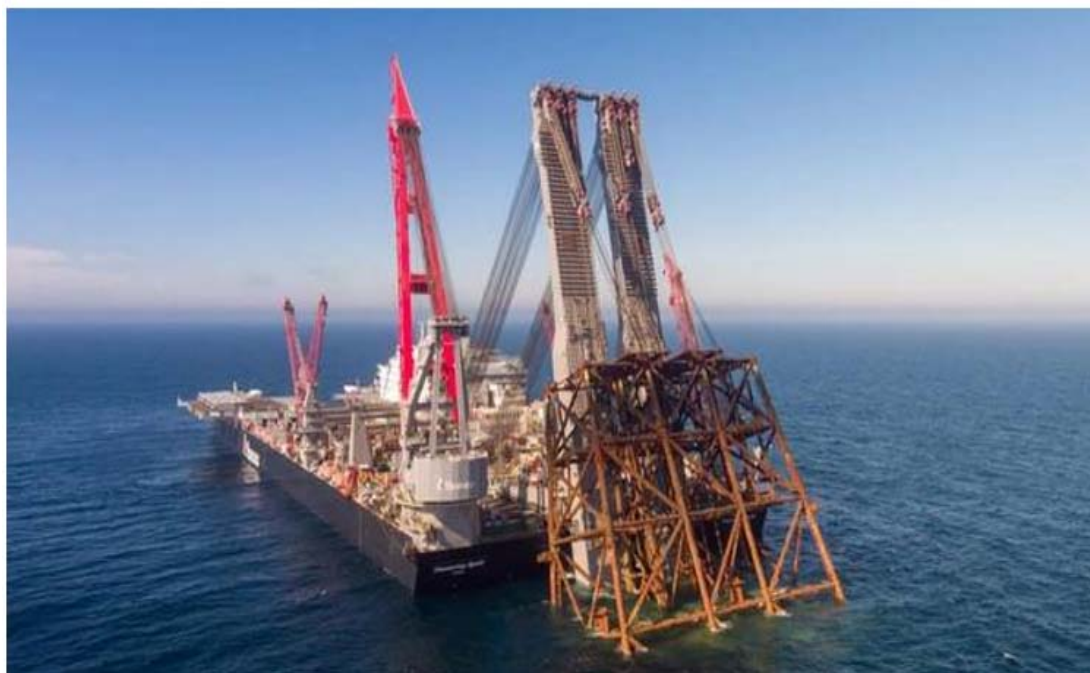
Figure 2: Pioneering Spirit Removing the Ninian Jacket (Source, Allseas)
