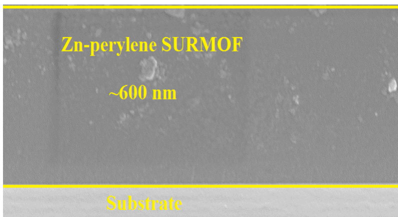
Fig. 2: Scanning Electron Microscope Showing the Thickness of Zn-perylene MOF thin film.
